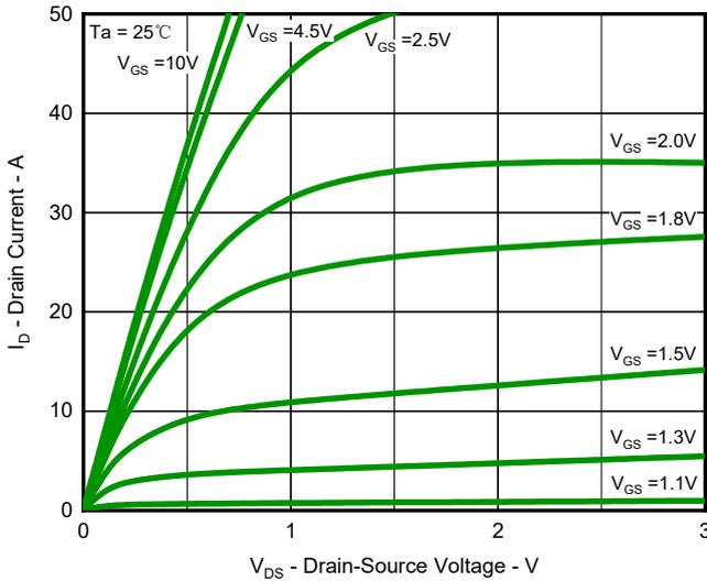
Fig.1 Output Characteristics
