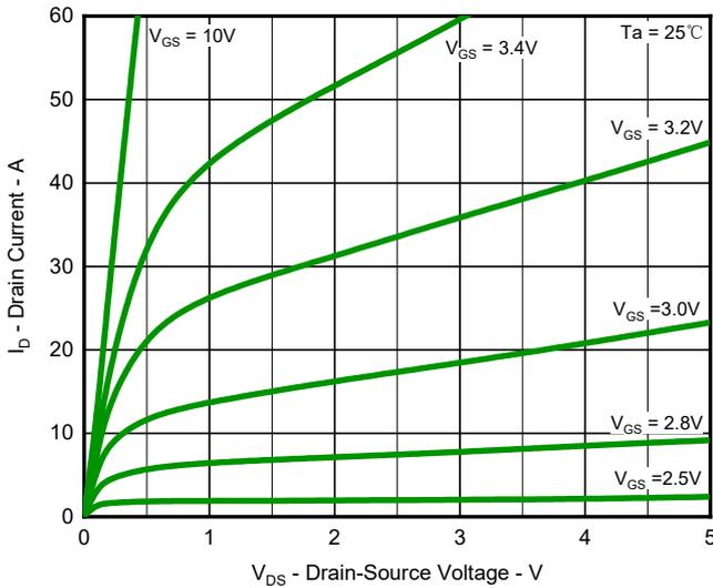
Fig.1 Output Characteristics
