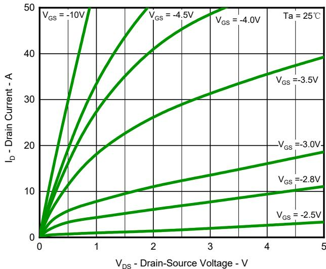
**Fig.1 Output Characteristics**
