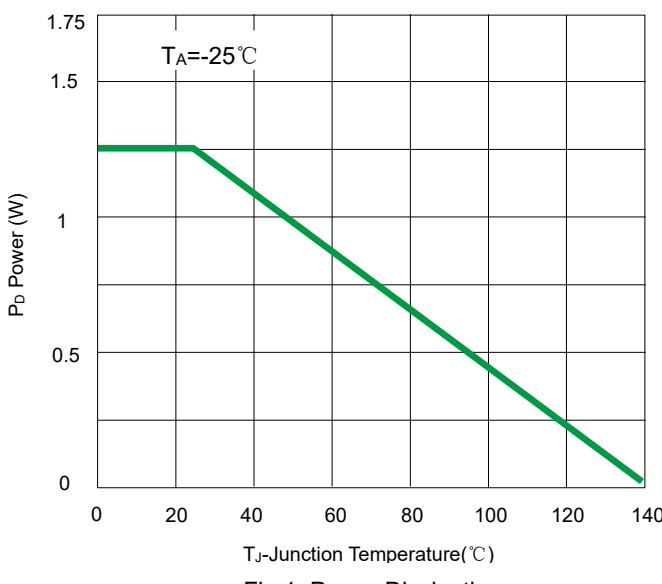
Fig 1. Power Dissipation
