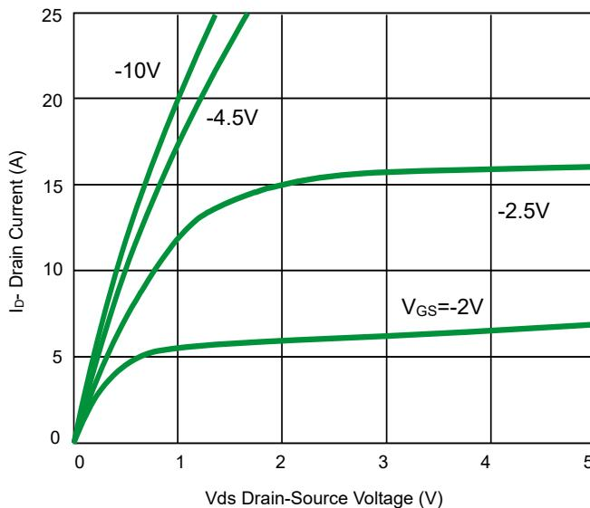
Fig 3. Output Characteristics
