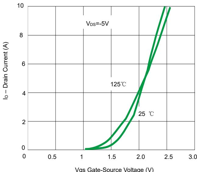
Fig 5. Transfer Characteristics
