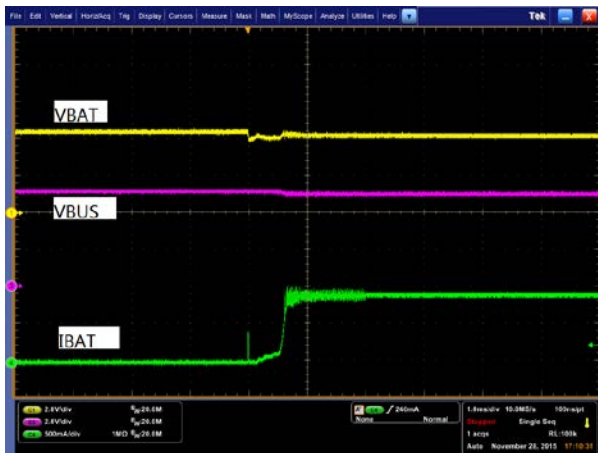
Figure 13. Battery Removal / Insertion during Charging, V_{BAT}=3.9V , I_{OCHARGE}=956mA , No I_{NLIM} , TE=0
