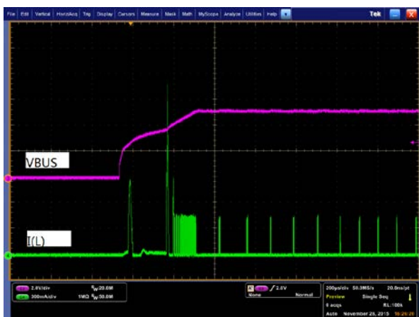
Figure 27. Startup, 3.6VBAT, 44Ω Load, Additional 10μF, X5R Across VBUS
