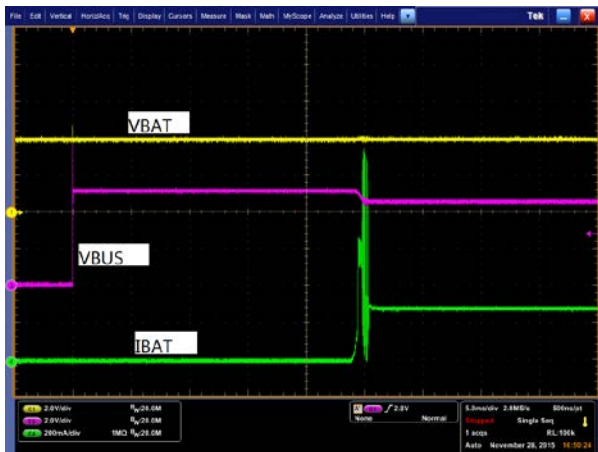
Figure 11. Auto-Charge Startup with 300mA Limited Charger/Adaptor, I_{NLIM}=500mA , V_{BAT}=3.9V
