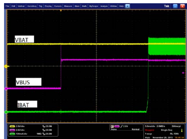
Figure 10. Auto-Charge Startup at V_{BUS} Plug-in, I_{INLIM}=500mA , V_{BAT}=3.9V
