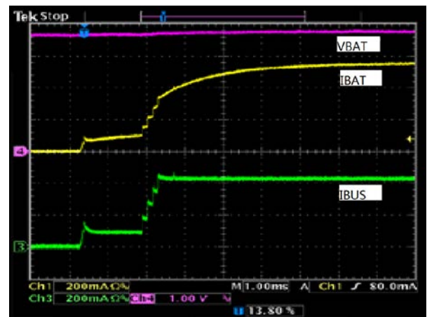
Figure 12. Charger Startup with HZ_MODE Bit Reset, I_{NLIM}=500mA , I_{OCHARGE}=956mA , O_{REG}=4.2V , V_{BAT}=3.6V
